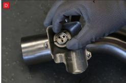
B) After you have removed O.E exhaust you will need to swap the valve motor to the Scorpion exhaust. Remove the 3 nuts ( keep safe as you will need them to bolt the electronic valve motor to Scorpion Exhaust).
